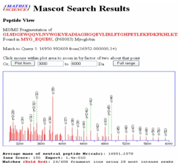
Figure 8: Results of the MASCOT Software MS/MS Ion Search for the ISD spectrum of Myoglobin. To obtain this result, the intact mass of the protein was determined from MS mode analysis, and then this measured mass was used in the MS/MS ion type search.
